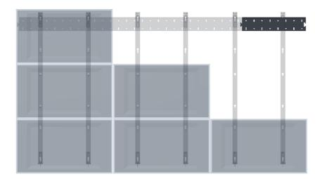
**VWM-MA-?-?**, Monitor mounting arms suitable for 1, 2 or 3 stacked monitors. The type of MA arm is determined by the diagonal and screen height.
