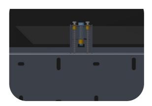
Use the M8 to only adjust the height of the upper monitor.
