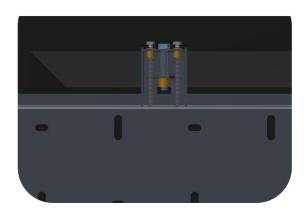
Use the M6 screws to level out the total MA arm on the BPH.
