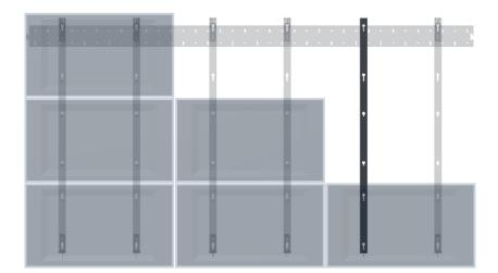
The monitors are being installed with the by Audipack provided special mounting cams. These cams can be inserted at the back of the monitors. There are several cams available with different thread dimensions.
