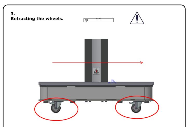
To retract the wheels it is importand to have the wheels positioned in the correct direction. All wheels are detected by the electrical system and allow the system to descend.
