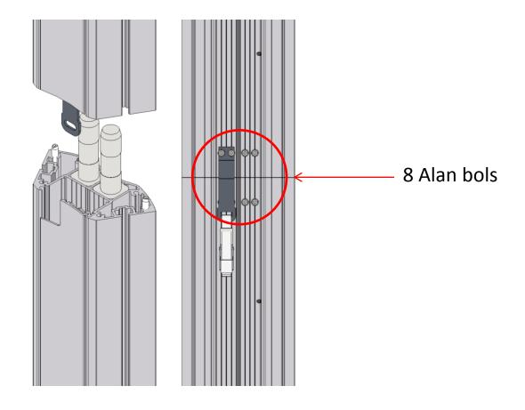
A column extension or relacement needs an alignment check before setting up the columns together. Because columns are made from different production badges it might be possible the stand will not fit right the first time.
