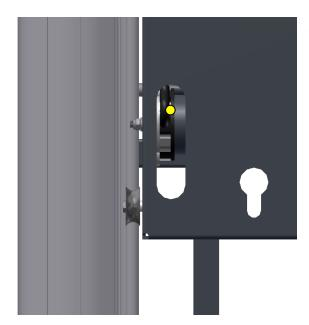
At the front of the lifting head colored knobs are visible. With an alan key the positions can be set by adjusting their position.
