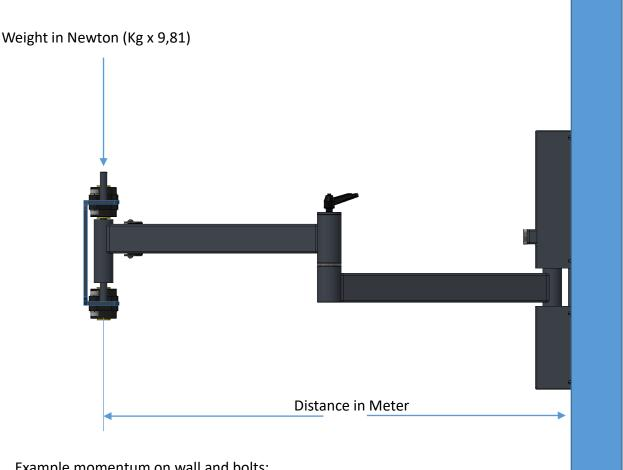
Example momentum on wall and bolts: 100 Kg x 9,81 x 1,05 meter = 1030 Nm
