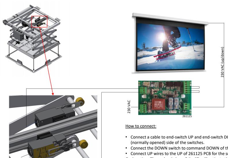
Connect a cable to end-switch UP and end-switch DOWN to the NO
