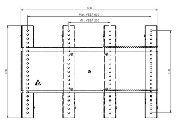
Max. load: 85 kg L&S5 mounting interface is a registered product Dimensions are indications, not to be used for any preparations. No rights can be derived from the above dimensions.
