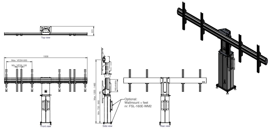
Power supply : 230 VAC Maximum load 85 kg Maximum screen size : 55 inch
