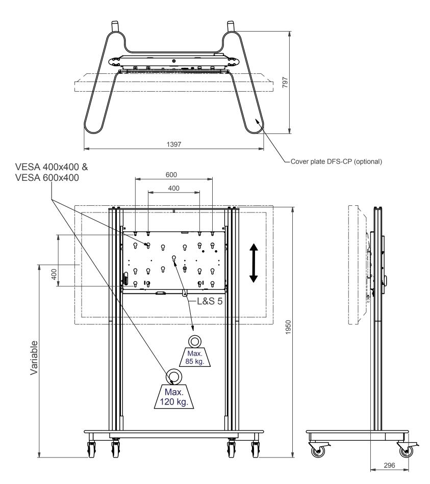
Power supply 230 volt Max. load 120 Kg Standard :L&S5 mounting interface RF remote controlled
